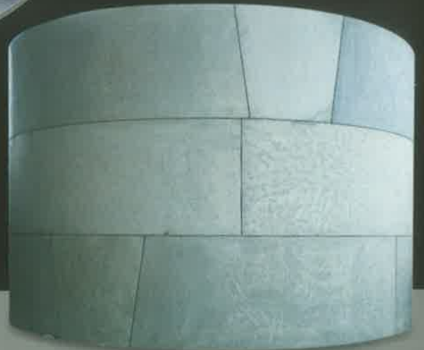
Assembling of Master Ring For Dimensional Checking
